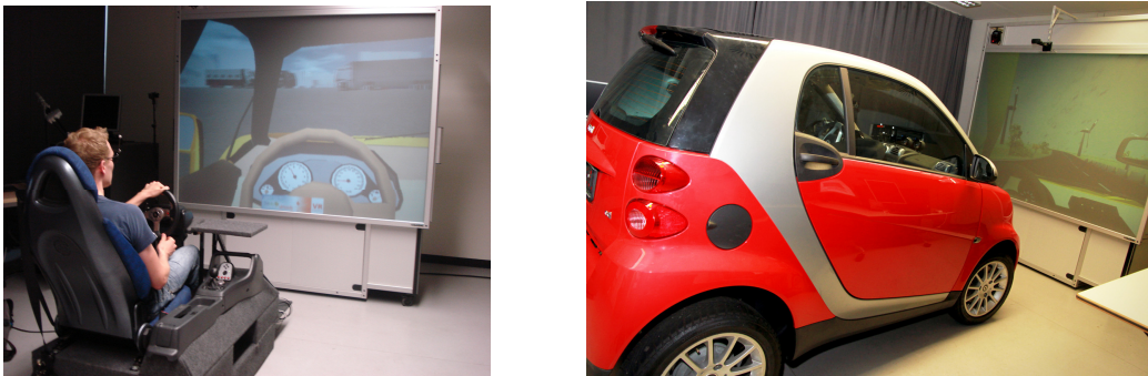
Fig. 3. (a) First prototype of DRIVE project in MR lab; (b) Second prototype of DRIVE project using real car as input device
